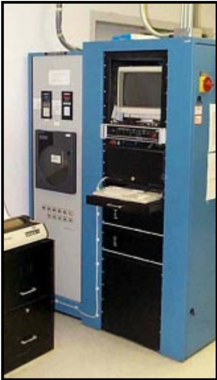
Photo 2 —The environmental chamber is computer controlled. Temperature and vibration profiles are programmed for the entire test sequence and run without supervision.
