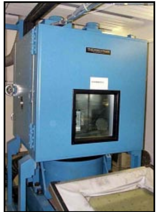
Photo 1 —This is the torture chamber for temperature, vibration, and humidity testing. Notice the slip table in front of the chamber. This, in conjunction with the cylindrical driver under the chamber, provides vibrations in all three axes.
