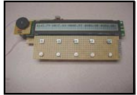
Photo 1—Under the LCD is a socketed 68HC11F1, and the other supporting components. The dial is a contrast control which come assembled to the LCD.
